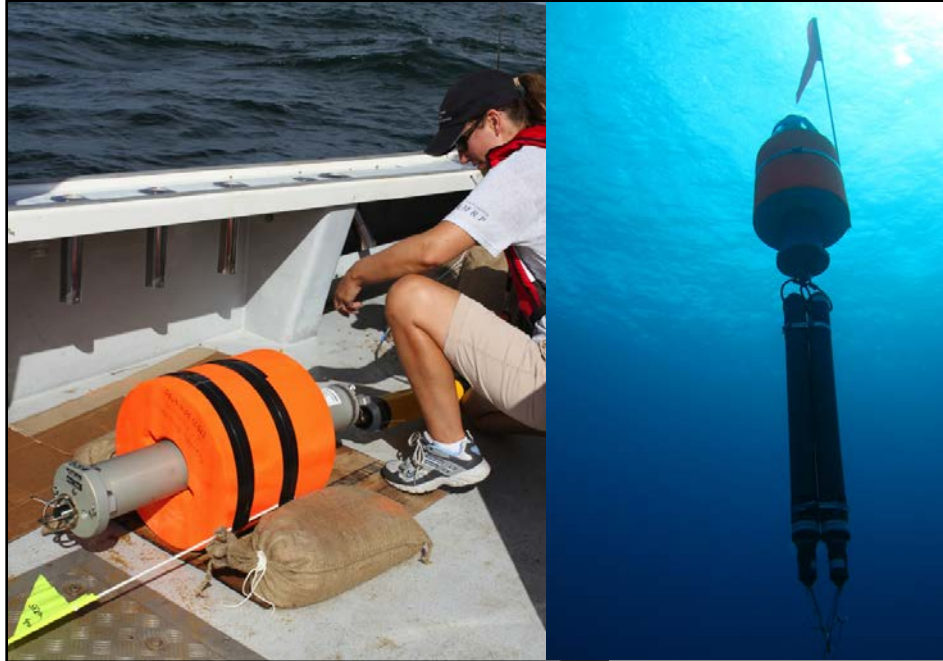
Figure 2. Images of an EAR prior to deployment and while deployed.
